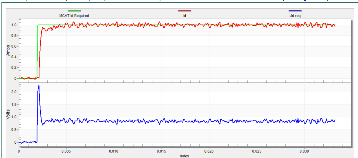
Figure 51. Optimal step response of the Id current controller
