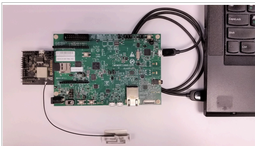
Figure 16. i.MX RT1060 EVK connection to the host computer for power supply and console access
