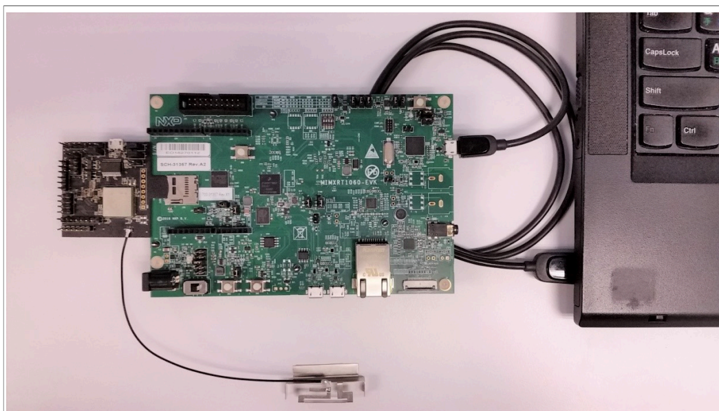
Figure 15. i.MX RT1060 EVK connection to the host computer for power supply and console access
